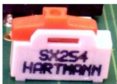
Switch position left (delivery status)
